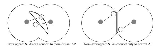
Figure 2 - Overlapped and Non-Overlapped BSA Coverage
